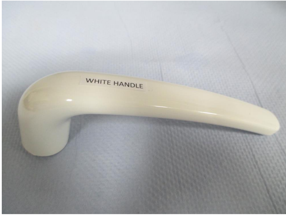
Photograph showing the condition of the White Handle Sample prior to Salt Spray Test
