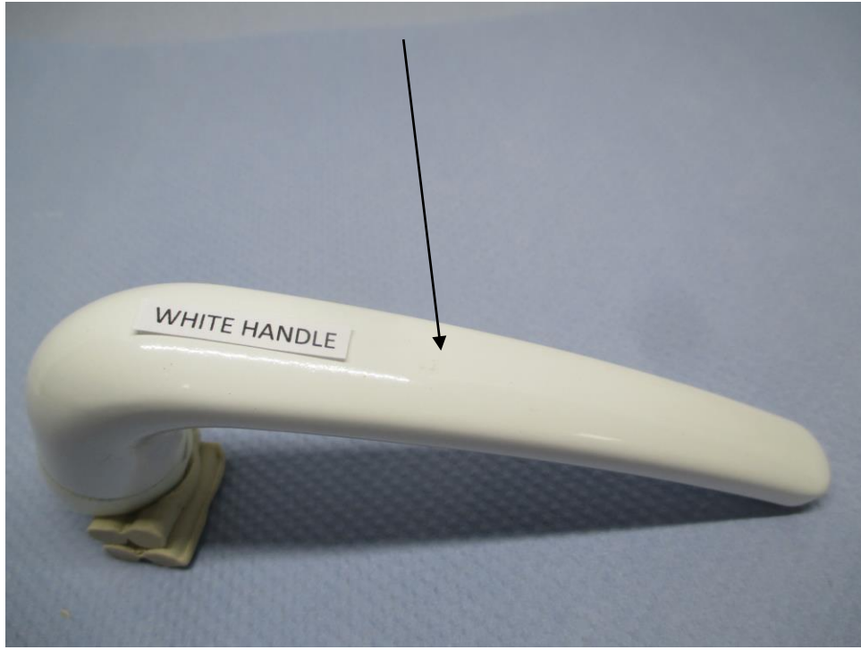
Photograph showing the condition of the White Handle Sample after 480 hours Salt Spray Test
