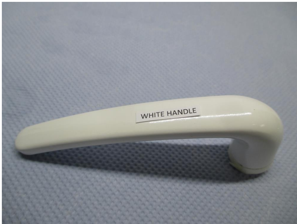
Photograph showing the condition of the White Handle Sample after 96 hours Salt Spray Test
