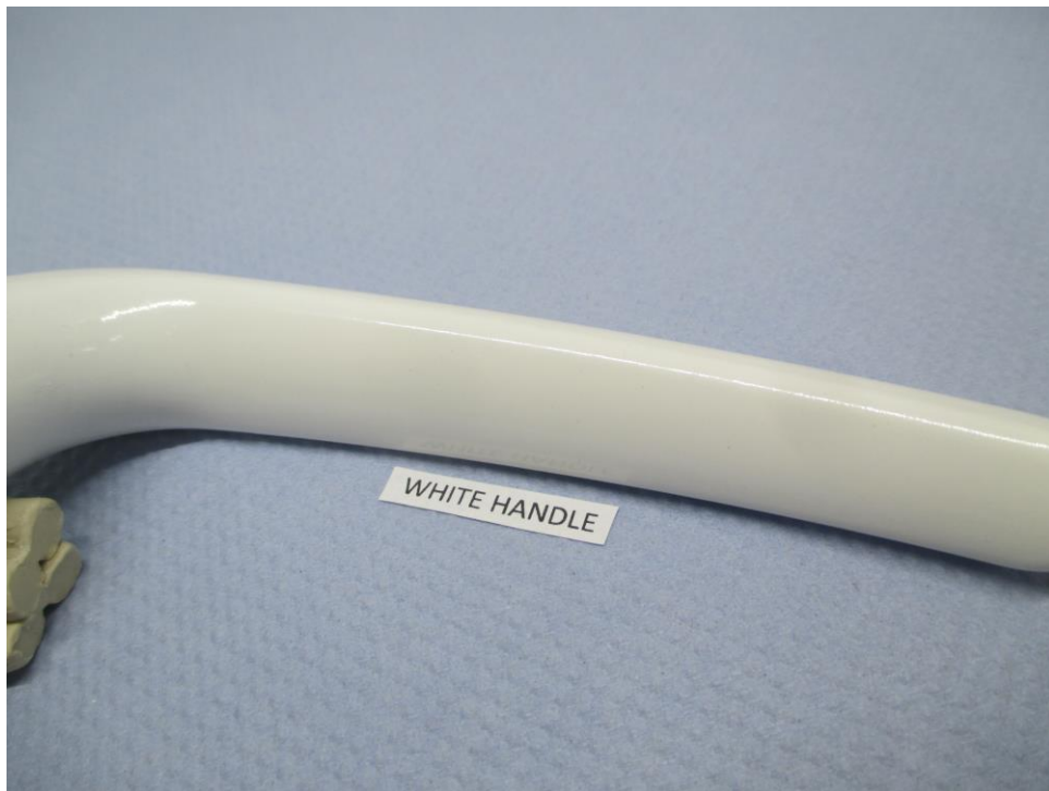
Photograph showing the condition of the White Handle Sample after 1008 hours Salt Spray Test
