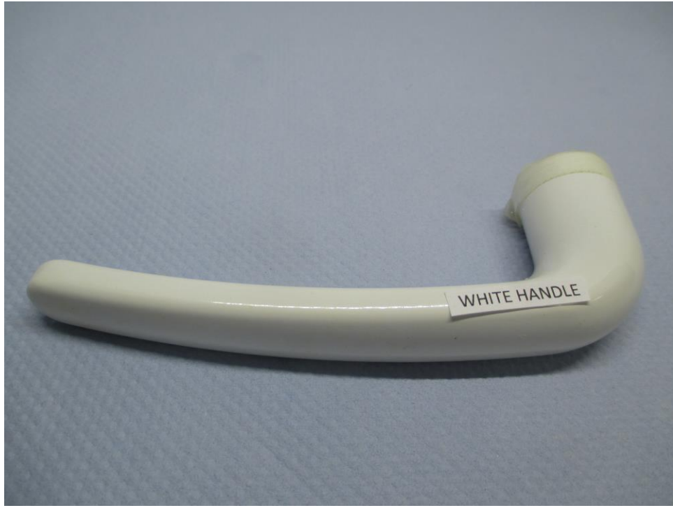
Photograph showing the condition of the White Handle Sample after 264 hours Salt Spray Test
