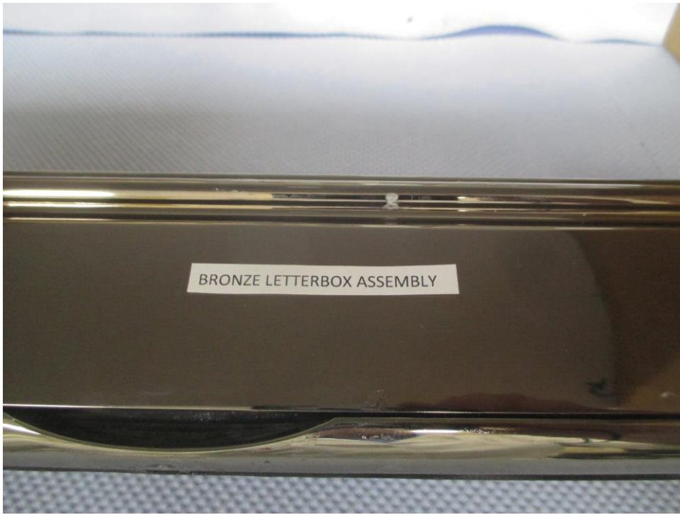
Photograph showing the condition of the Bronze Letterbox Assembly after 96 hours Salt Spray Test
