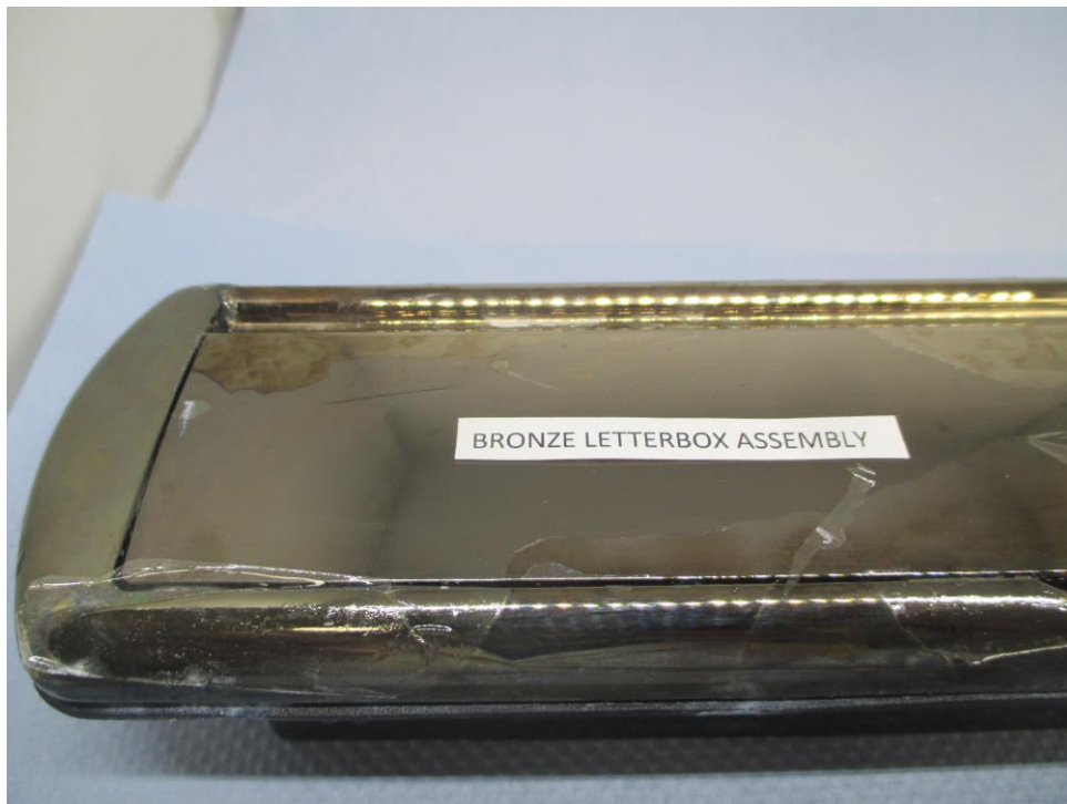
Photograph showing the condition of the Bronze Letterbox Assembly after 1008 hours Salt Spray Test
