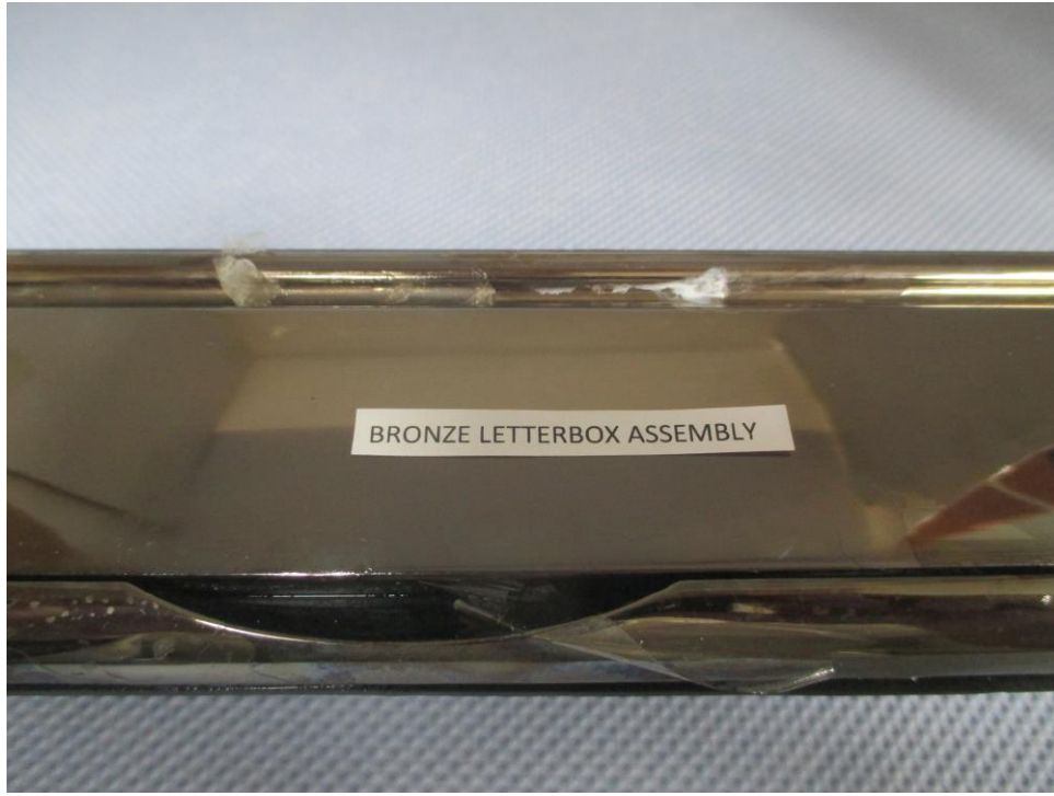
Photograph showing the condition of the Bronze Letterbox Assembly after 480 hours Salt Spray Test
