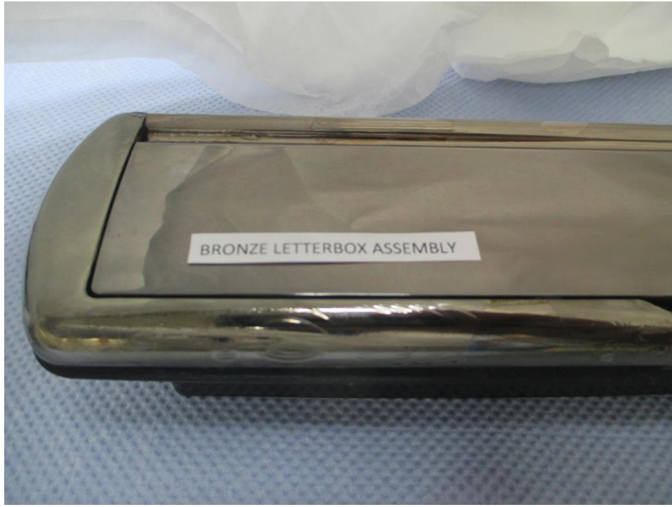
Photograph showing the condition of the Bronze Letterbox Assembly after 264 hours Salt Spray Test
