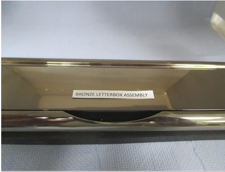
Photograph showing the condition of the Bronze Letterbox Assembly prior to Salt Spray Test
