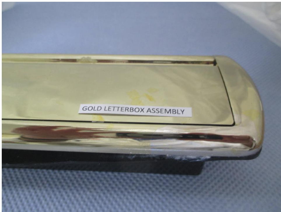
Photograph showing the condition of the Gold Letterbox Assembly after 264 hours Salt Spray Test
