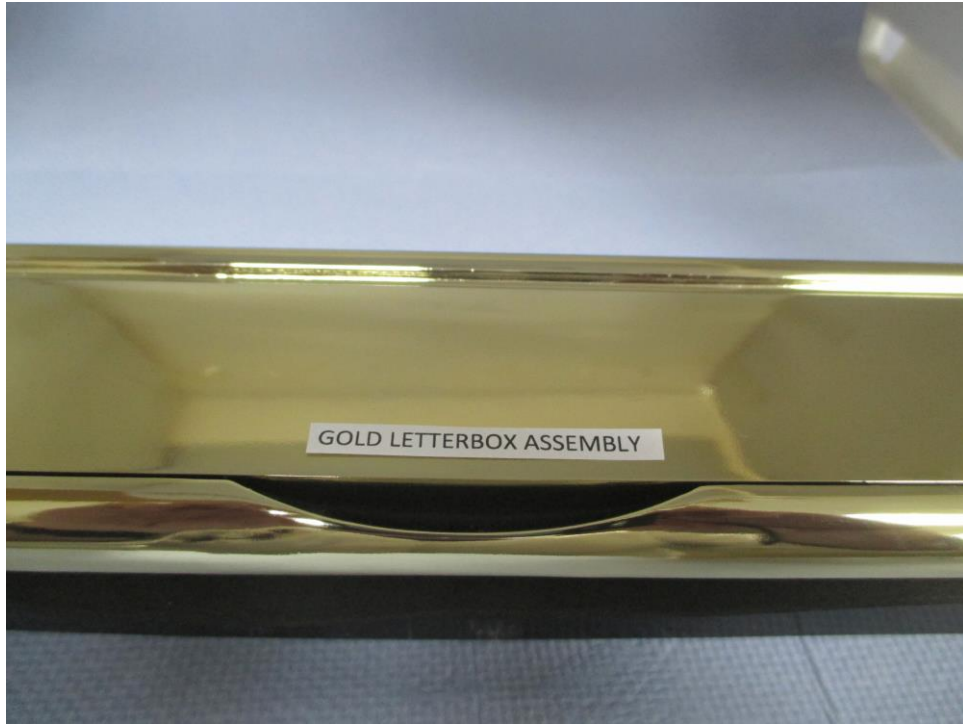
Photograph showing the condition of the Gold Letterbox Assembly prior to Salt Spray Test
