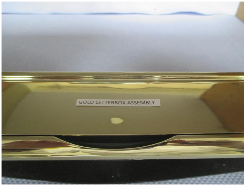
Photograph showing the condition of the Gold Letterbox Assembly after 96 hours Salt Spray Test
