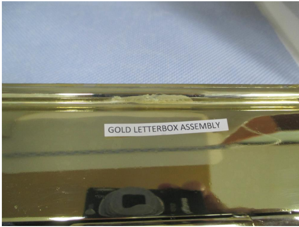
Photograph showing the condition of the Gold Letterbox Assembly after 480 hours Salt Spray Test
