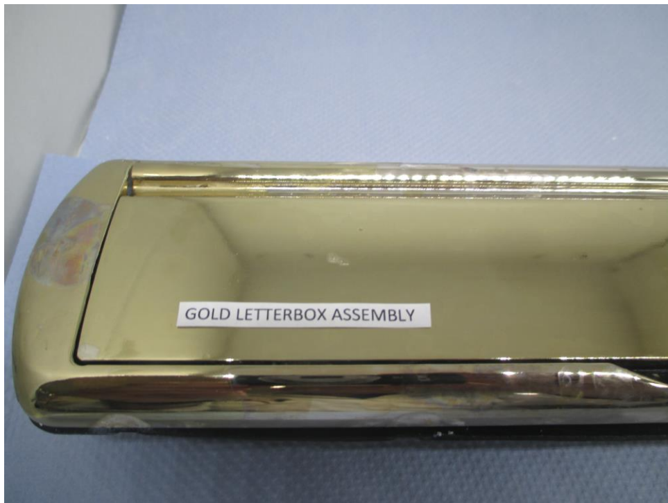
Photograph showing the condition of the Gold Letterbox Assembly after 1008 hours Salt Spray Test
