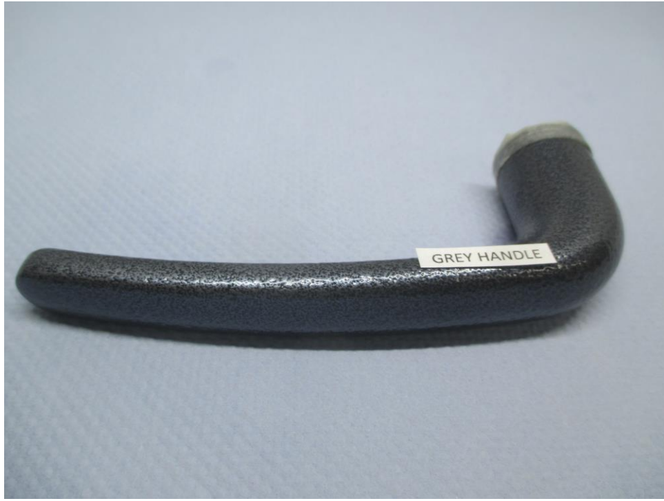
Photograph showing the condition of the Grey Handle Sample after 264 hours Salt Spray Test
