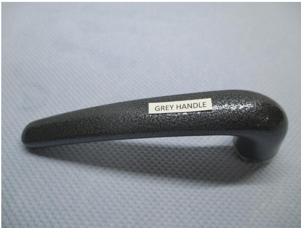
Photograph showing the condition of the Grey Handle Sample after 96 hours Salt Spray Test
