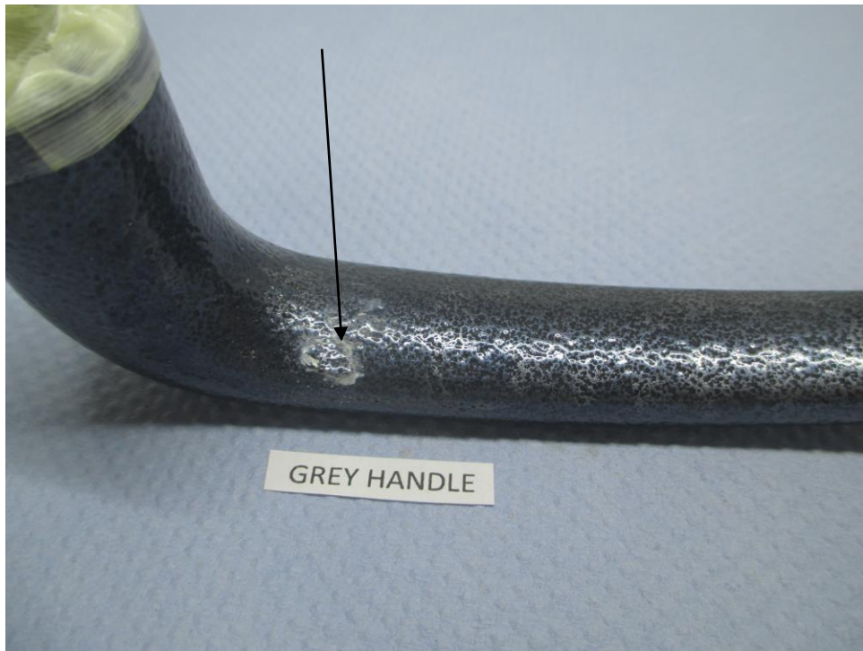
Photograph showing the condition of the Grey Handle Sample after 1008 hours Salt Spray Test (Damaged area)
