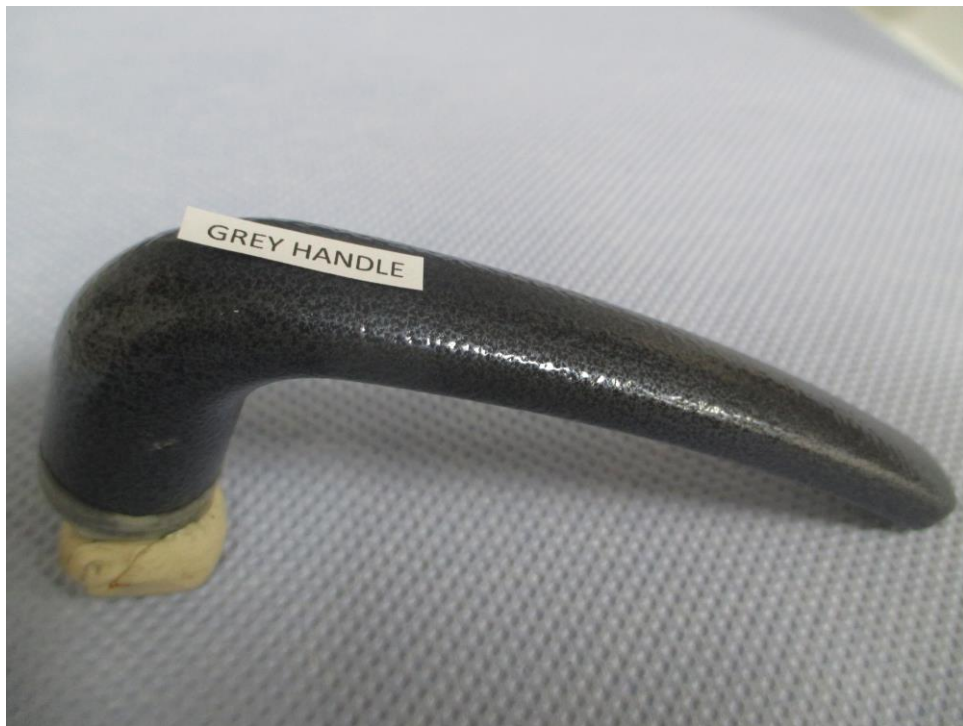
Photograph showing the condition of the Grey Handle Sample after 480 hours Salt Spray Test
