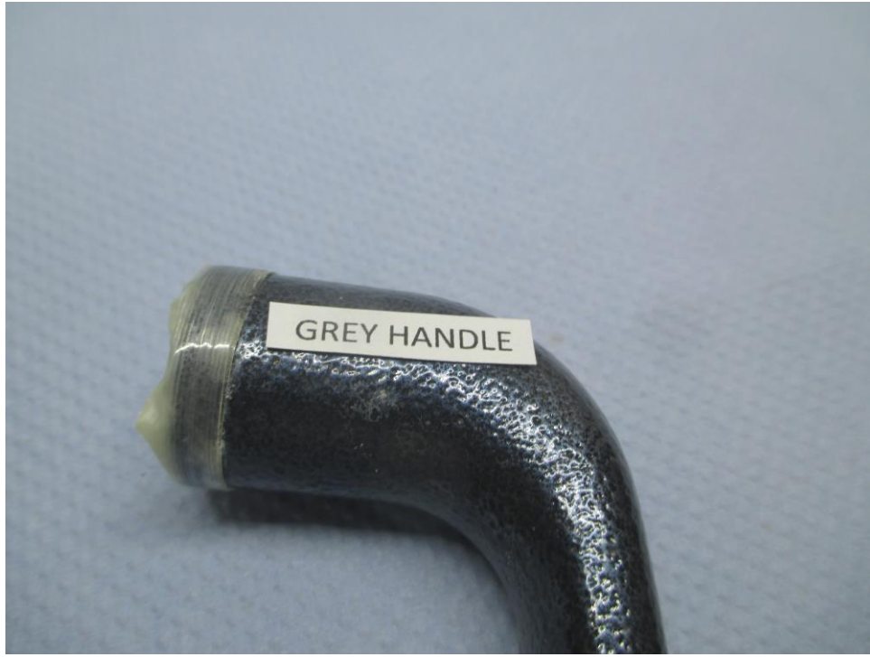
Photograph showing the condition of the Grey Handle Sample after 1008 hours Salt Spray Test
